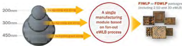
Figure 2: FlexLine™ seamlessly processes multiple silicon wafer diameters on the same manufacturing line to produce both FIWLP and FOWLP.
