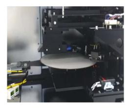
**Figure 6.** Pre-aligner station where the wafer notch is detected and wafer ID is read of eWLCSP carrier in prober system in FlexLine
