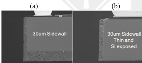
Figure 5. SEM micrographs of cross-section of: (a) eWLCSP™ and (b) thin eWLCSP™.
