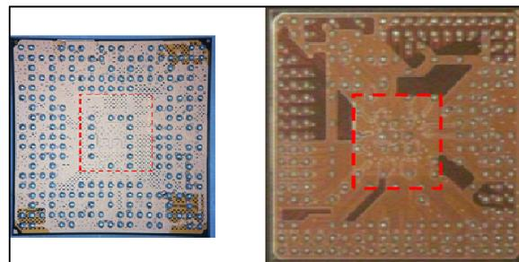
Figure 5: Micrograph of 10mm x 10mm and 13mm x 13mm packages; outline of approximate position of the die are shown as the red dotted box.
