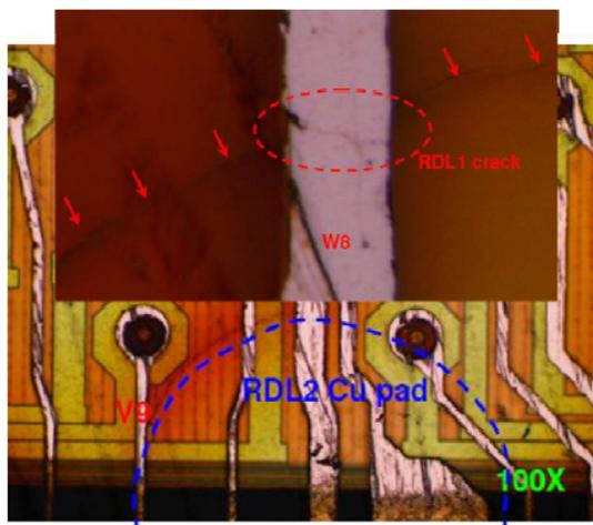
Figure 7: Micrographs representative of all 13mm x 13mm TCB induced failures.
