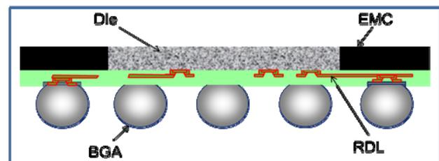
Figure 1: Schematic of an exposed die FO-WLP
