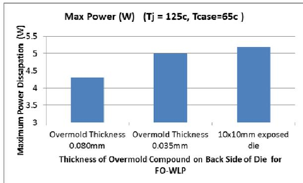
Figure 2: Dependence of max power dissipation on mold thickness on back side of die in a 10mm x 10mm FO-WLP
