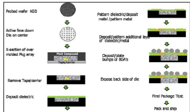
Figure 3: Overview of process flow for the devices used in this work
