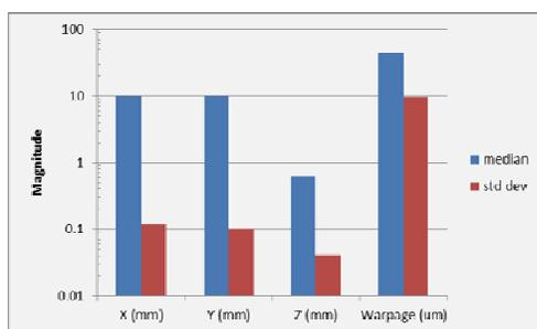
Figure 6: Median and standard deviation of X, Y, and Z dimensional control and of final package warpage at room temperature for the 10mm x 10mm package
