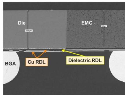
Figure 4: Cross section of a 13x13mm FO-WLP test vehicle
