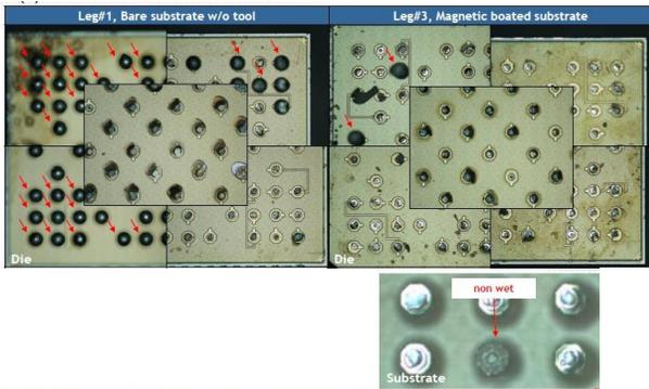
Figure 7: Examples of severe non-wet w/ coreless substrate using magnetic boat, and tape carrier on all substrate types except “control”
